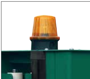
Flashing warning light A safety precaution to prevent accidents
